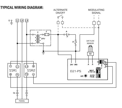
To switch the input between 0-10 VDC and AC/DC pulse, simply remove and replace the jumper according to the label. D21-PS controllers may be used to drive up to 4 SSRs. The maximum load is limited to the capacity of the Solid State Relays. In cases with smaller loads, consider the D21-P with a single output and the D22-P equipped with two outputs effectively doubling the capacity of the D21-P.
