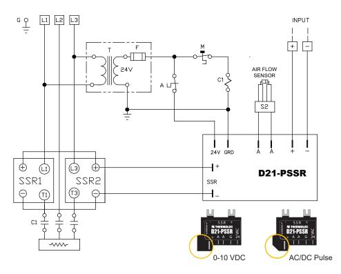
The board is factory set for either 0-10 VDC or AC/DC pulse. D21-PSSR controllers may be used to drive up to 2 SSRs. For driving 4 SSRs the D21-PS is required. The maximum load is limited to the capacity of the Solid State Relays. In cases with smaller loads, consider the D21-P with a single output and the D22-P equipped with two outputs effectively doubling the capacity of the D21-P.
