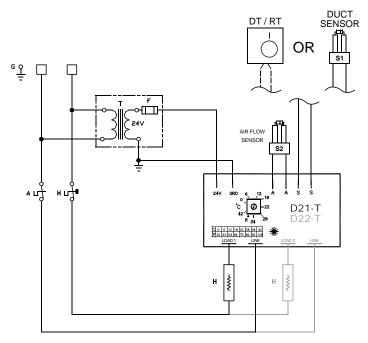
Thermolec's RTs and DTs are available in a variety of temperature ranges. Please order the proper range for your application The D21-T has a single output with a maximum load as listed in the table below. The D22-T is equipped with two outputs effectively doubling the capacity of the D21-T. In cases with even larger loads, a D21-TS may be used instead to drive up to 4 SSRs. The maximum load is then limited to the capacity of the Solid State Relays.
