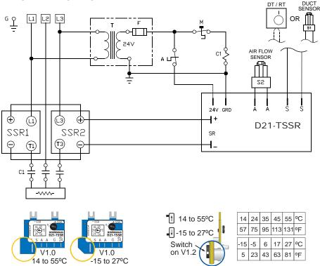
Thermolec's RTs and DTs are available in a variety of temperature ranges. Please order the proper range for your application. D21-TSSR controllers may be used to drive up to 2 SSRs. The maximum load is limited to the capacity of the Solid State Relays.
