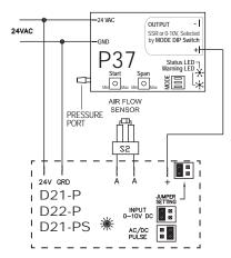
For use with D21-P, D22-P or D21-PS board set MODE SWITCH to 0-10 VDC and connect the positive output to the positive input on the D2x-P series board and place the jumper on the 0-10VDC position.
