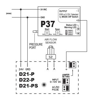
For use with D21-P, D22-P or D21-PS board set MODE SWITCH to 0-10 VDC and connect the positive output to the positive input on the D2x-P series board and place the jumper on the 0-10VDC position.
