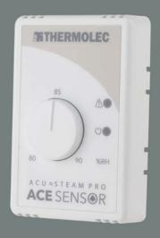
Thermolec's exclusive ACE SENSOR monitors the conditions in the duct to prevent excessive buildup of humidity. It is included with every AcuSteam Pro and may be used with the residential AcuSteam as an option. The high limit cutoff is adjustable from 80 to 90% RH.
