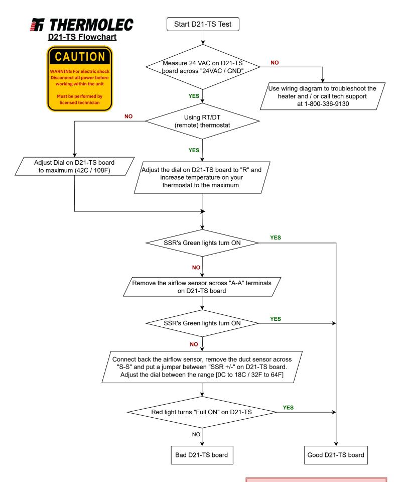
**NOTE:** Please put back connections and jumpers as per wiring diagram
