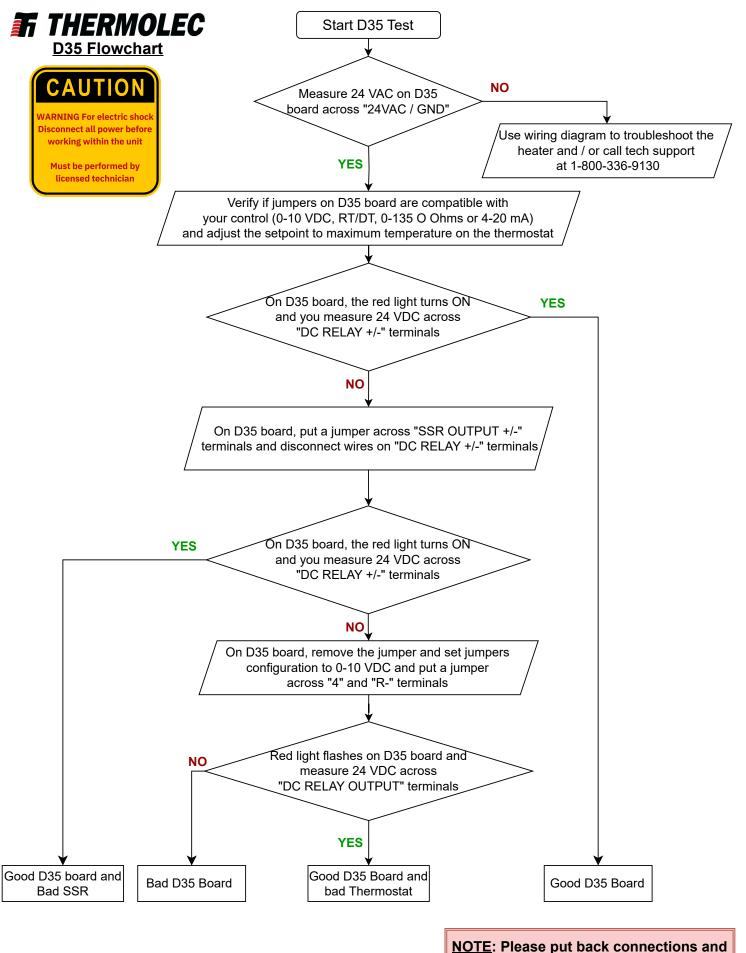
jumpers as per wiring diagram
