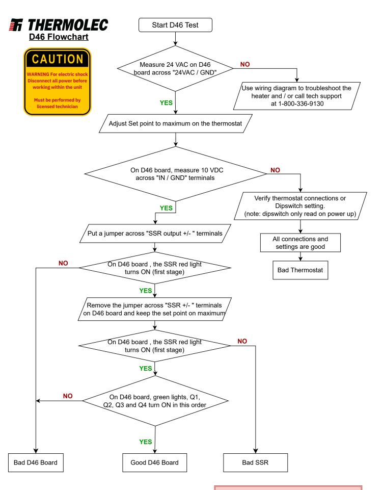
NOTE: Please put back connections and jumpers as per wiring diagram
