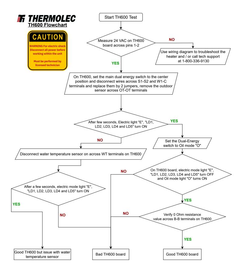
NOTE: Please put back connections and jumpers as per wiring diagram
